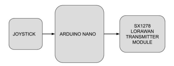
In this project we used Arduino Nano as a microcontroller. As an input device we used a joystick and as an output device the lorawan transmitter module.
