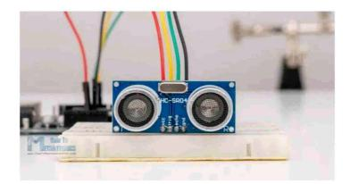
The high-frequency sound waves generated by active ultrasonic sensors are received back by the ultrasonic sensor for evaluating the echo. Thus, the time interval taken for transmitting and receiving the echo is used for determining the distance to an object. But, passive ultrasonic sensors are just used for detecting ultrasonic noise which is present under specific conditions.
