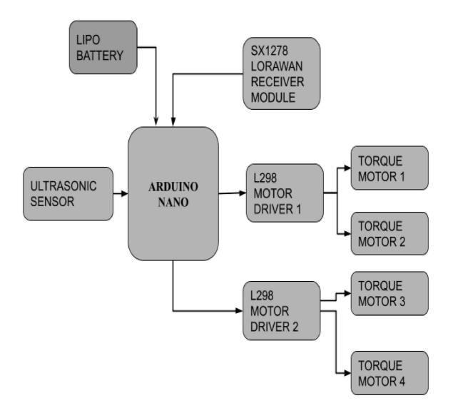
In this project we used Arduino Nano as a microcontroller. Ultrasonic is connected as an input device to the Arduino Nano. The 2 L298 motor driver is connected to the microcontroller as an output device. The 4 torque motor is attached SX1278 receiver lorawan module is connected as an input device to the arduino nano.
