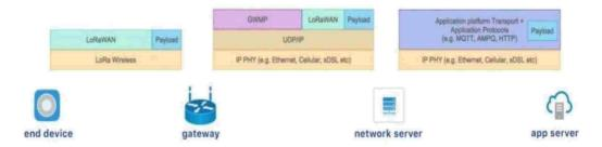
Gateways send LoRaWAN messages over the wireless interface using the gateway Message Protocol defined in accordance with the LoRaWAN Gateway to Server interface specification. LoRaWAN messages and attached data are sent in JSON encoded format using UDP/IP
